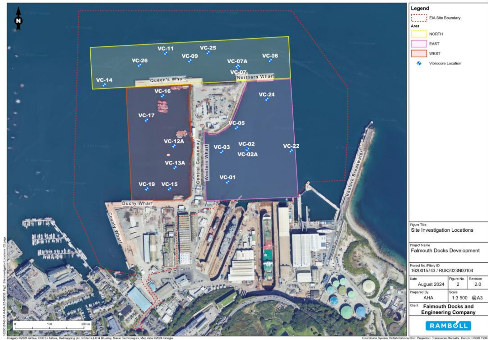
Figure 3: March 2024 Ground Investigation Vibrocore Locations
