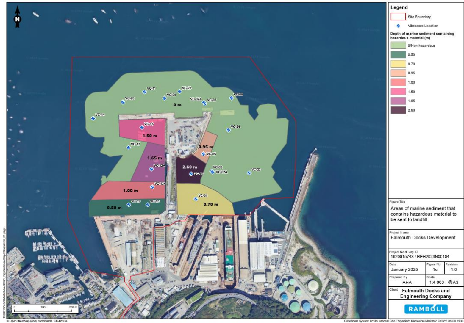
Appendix 3, Figure 1: Estimated Thickness of Shallow Sediments (Depth from Seabed Surface) Considered to be Hazardous
